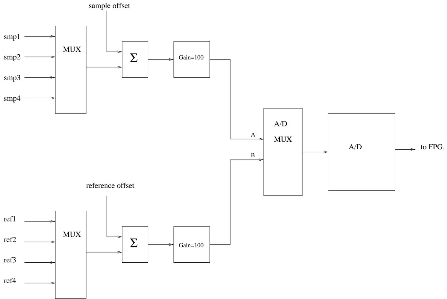
Fig. 2 A/D input connections
