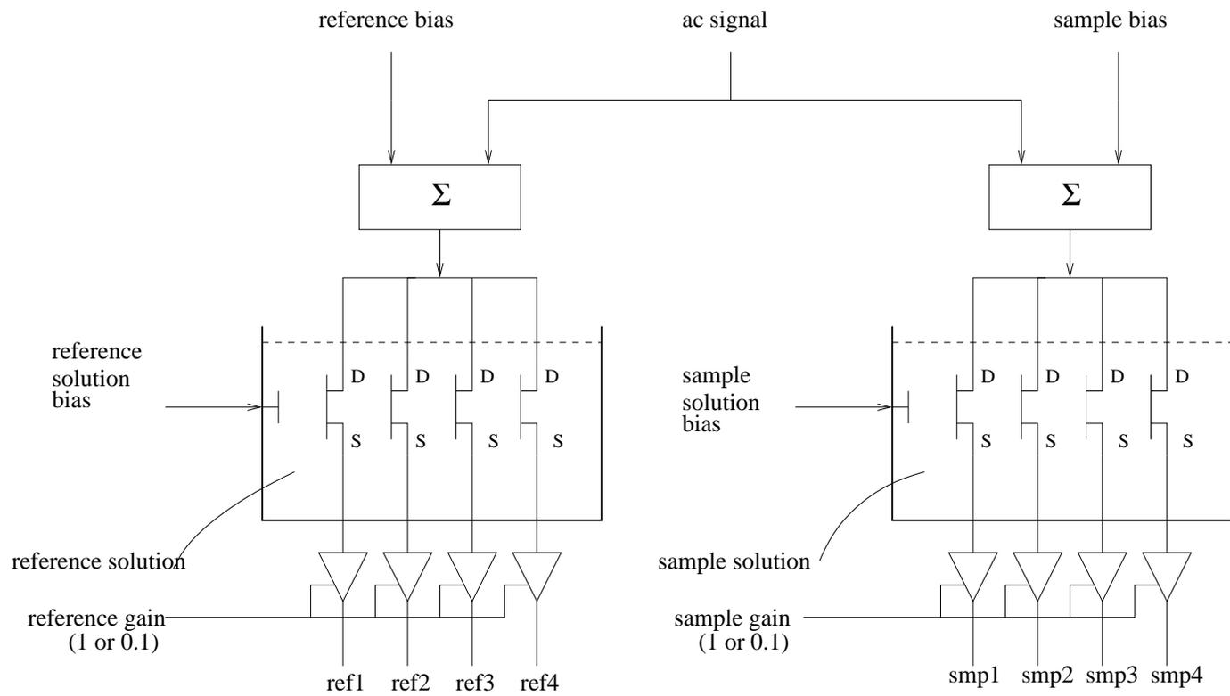
Fig. 1 Bio-sensor electrical connections
